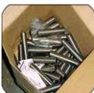
The contents move freely causing damage to the package. Cargo needs To be properly blocked and braced with dunnage to prevent movement inside the package. ALL voids To be filled when transporting cargo in corrugated fiberboard boxes.
